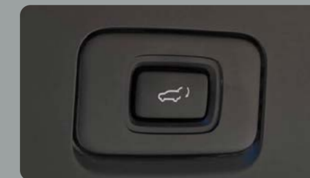
Remotely-triggered Power lift gate with step sensor and control switch** with buttons on the smart key, inside the cabin and on the lift gate**.
