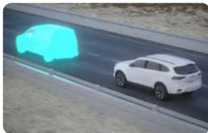
FORWARD COLLISION WARNING [FCW]: Your ISUZU D-MAX alerts you when an obstacle is detected in your path, sounding an audible alert and displaying a visual, heads-up windscreen warning.
