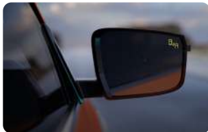
BLIND SPOT MONITOR [BSM]: Your ISUZU D-MAX displays a visual warning in your side mirrors when a vehicle approaches in your blind spot.
