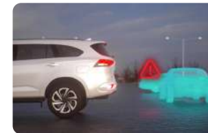
REVERSING CAMERA with REAR TRAFFIC ALERT [RCTA]: Monitors your surrounding area while reversing into traffic, providing visual and audible warnings should an object approach from the left or right.
